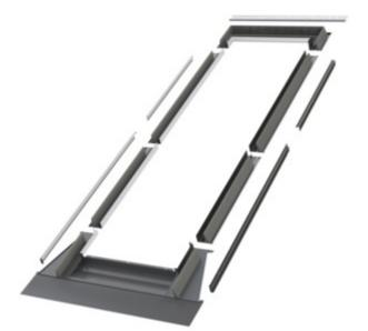
A sealing collar that allows a tight connection between a window and profiled roofing materials such as tiles, high profile sheeting. It can be used for roof coverings with a profile height of up to 90 mm.
