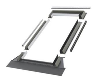
The flashing enables tight connection of a window with profiled roof coverings such as tiles and high profile metal sheeting. It can be used for roof coverings with a profile height of up to 90 mm.
